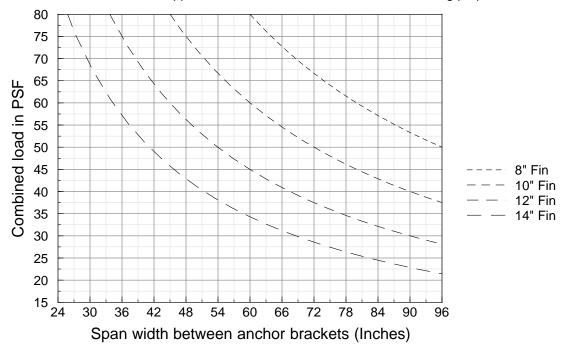
For twin span bracket applications CW backmember must also be engineered to account for overall system load
